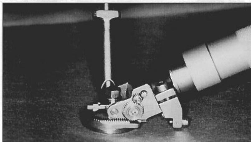
Figure 2. The assembled microkeratome, engaged in the dovetail guide of the suction ring.
