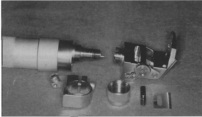
Figure 4. Disassembled microkeratome.
