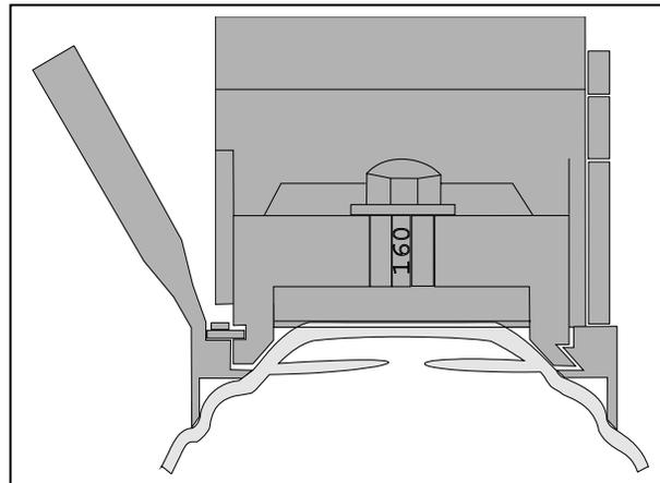
**Fig. 7(b).** Cross-sectional diagram showing how the microkeratome cuts a lamellar section through the cornea by flattening the central corneal area.
